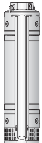
Reinforced with special collar from Collar especial de refuerzo de 6SDX(L) 13/33
